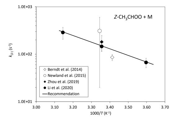
Arrhenius plot of  $k_{(Z-)}$ . Direct determinations are shown as filled points; relative rate determinations are shown as open points. The displayed errors are the experimental limits cited by the authors (but do not include uncertainty in the reference reaction for the relative rate studies). The line is the IUPAC recommendation,  $k_{(Z-)} = 7.4 \times 10^6 \text{ exp}(-3220/T) \text{ s}^{-1}$ .
