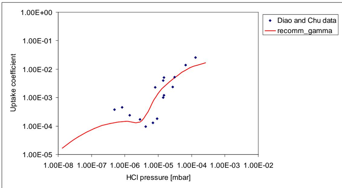
Figure 1: The recommended parameterization for the  $p(\text{HCl})$  dependence of the uptake coefficient of HONO on ice in the presence of HCl (red line), along with the data by Diao and Chu (2005).
